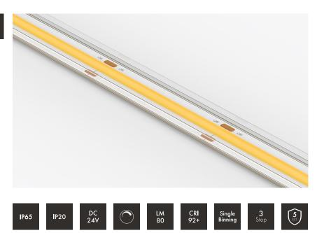
Our COB ULTRA RUN Series are designed to offer a dotless Linear finish in applications which require extra long lighting runs but are constrained by limited power outlets. Our 5W per metre model features 480 SMD LEDs, self regulating IC resistors and an extra thick 30z PCB board for a durable finish.
