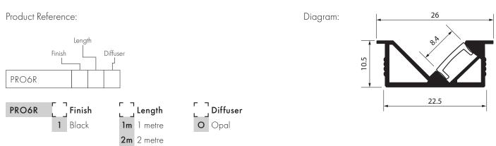
Each metre of fossLED profile comes with two End Caps (one with and one without a cable feed hole) as standard; for extra accessory packs please quote code PRO6R-1AC.
