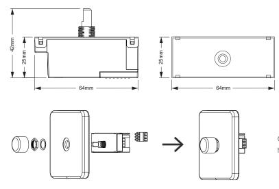
Compatible with traditional faceplates, simply replace the existing dimmer module as shown below.
