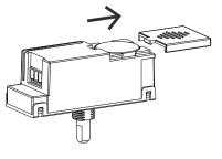
Please remove the protective film on the CR2032 battery before the first use.
