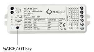
Match: After the receiver is powered on, short press the MATCH/SET Key on the receiver, immediately short press the knob (a) or rotate the knob **b**, the **LED indicator** flashes fast meaning the controller is successfully paired.
