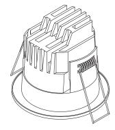
Adjust the tilt angle / direction as desired from above or below the fixture depending on access.
