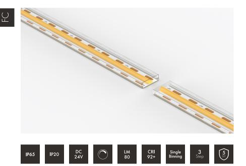
Our FREE CUT COB Series Strips are designed to offer a dotless Linear finish and be customised to precise lengths; feel free to cut anywhere along the LED Strips PCB board for a millimetre perfect finish. This 5W per metre model features 480 SMD LEDs on a 20z PCB board for a durable finish.
