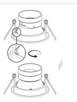
Fit the fixture into the ceiling by aligning the tabs and then rotating the inner cup until tight.
