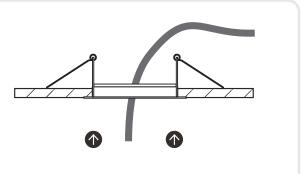
Push the springs upwards and fit into the ceiling hole ensuring the product is string properly and no cables are trapped.
