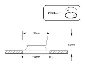
When installed in conjunction with our 'Insulation bracket' (Sold Seprately) this product is suitable for coverage by thermal and acoustic insulation e.g. loft insulation. Not suitable for blown insulation. Please ensure a max wattage of 7W when covering with insulation and utilising the insulation bracket.
