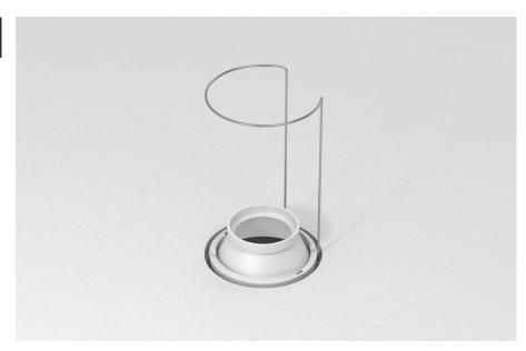
The Insulation Guard creates an airgap between a light fixture and the insulation, allowing compatible downlights to be covered by thermal and acoustic insulation e.g. loft insulation. Not suitable for blown insulation.
