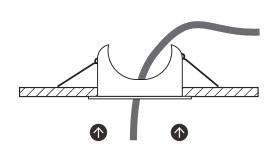
Push the springs upwards and fit into the ceiling hole ensuring the product is stting properly and no cables are trapped.
