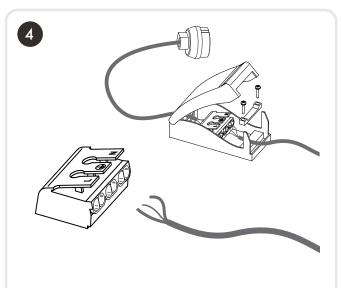
When wiring please ensure you have identified the correct wiring from the circuit and ensure the connections are tight and no loose strands have been left outside of the connection block.
