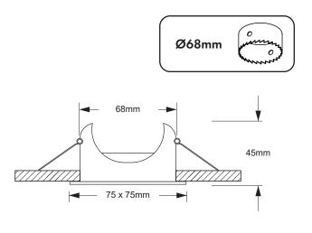
When installed in conjunction with our 'Insulation bracket' (Sold Seprately) this product is suitable for coverage by thermal and acoustic insulation e.g. loft insulation. Not suitable for blown insulation. Please ensure a max wattage of 10W when covering with insulation and utilising the insulation bracket.
