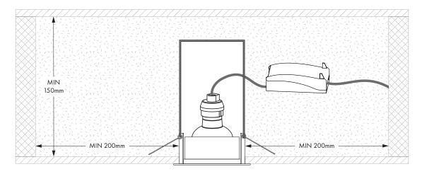
If installing without an insulation bracket please ensure any insulation is at a minimum distance of 150mm away from the fixture / lamp and not covering it.
