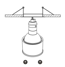
Fit by simply pushing the fixture into the ceiling making sure it is axially aligned.
