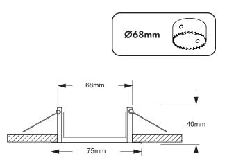
When installed in conjunction with our 'Insulation bracket' (Sold Seprately) this product is suitable for coverage by thermal and acoustic insulation e.g. loft insulation. Not suitable for blown insulation. Please ensure a max wattage of 7W when covering with insulation and utilising the insulation bracket.
