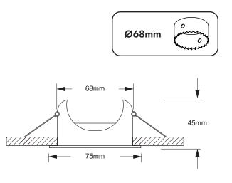
When installed in conjunction with our 'Insulation bracket' (Sold Seprately) this product is suitable for coverage by thermal and acoustic insulation e.g. loft insulation. Not suitable for blown insulation. Please ensure a max wattage of 10W when covering with insulation and utilising the insulation bracket.
