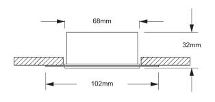
When installed in conjunction with our 'Insulation bracket' (Sold Seprately) this product is suitable for coverage by thermal and acoustic insulation e.g. loft insulation. Not suitable for blown insulation. Please ensure a max wattage of 7W when covering with insulation and utilising the insulation bracket.
