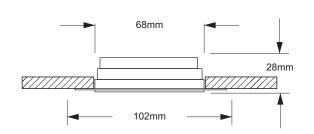
When installed in conjunction with our 'Insulation bracket' (Sold Seprately) this product is suitable for coverage by thermal and acoustic insulation e.g. loft insulation. Not suitable for blown insulation. Please ensure a max wattage of  $7\mathrm{W}$  when covering with insulation and utilising the insulation bracket.
