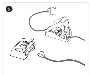
When wiring please ensure you have identified the correct wiring from the circuit and ensure the connections are tight and no loose strands have been left outside of the connection block.
