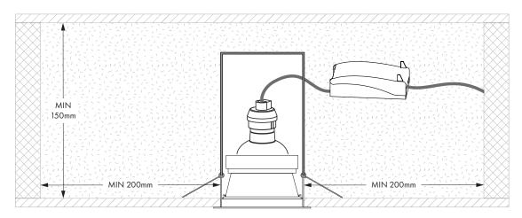
If installing without an insulation bracket please ensure any insulation is at a minimum distance of 150mm away from the fixture / lamp and not covering it.
