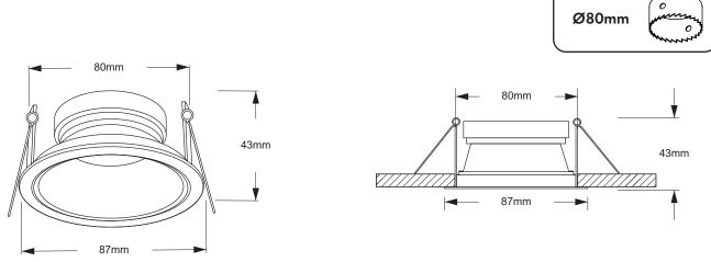
When installed in conjunction with our 'Insulation bracket' (Sold Seprately) this product is suitable for coverage by thermal and acoustic insulation e.g. loft insulation. Not suitable for blown insulation. Please ensure a max wattage of 7W when covering with insulation and utilising the insulation bracket.
