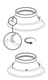
Fit the fixture into the ceiling by aligning the tabs and then rotating the inner cup until tight.
