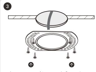
Screw a minimum of 6 screws to the fixture to keep it in place.
