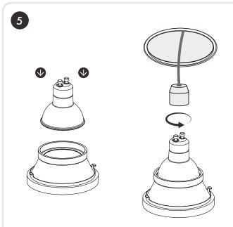
Fit the LED bulb into the fixture, then twist and connect your LED bulb.
