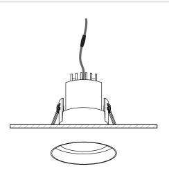
Connect the downlight to the connection block. Push the springs upwards and fit into the ceiling hole ensuring the product is sitting properly and no cables are trapped.
