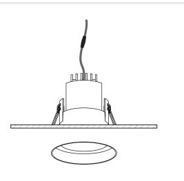
Connect the downlight to the connection block. Push the springs upwards and fit into the ceiling hole ensuring the product is sitting properly and no cables are trapped.
