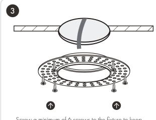
Screw a minimum of 6 screws to the fixture to keep it in place.
