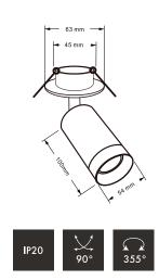
The Shooter L GU 10 Recessed - is a versatile recessed mounted spotlight fixture ideal for display and accent lighting purposes. This unit hosts a cylindrical base design, multi directional functions and a set back finish for reduced glare.
