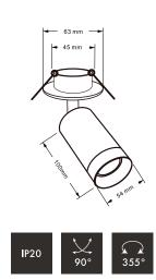
The Shooter L GU 10 Recessed - is a versatile recessed mounted spotlight fixture ideal for display and accent lighting purposes. This unit hosts a cylindrical base design, multi directional functions and a set back finish for reduced glare.
