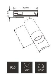
The Shooter L GU 10 - is a versatile track mounted spotlight fixture ideal for display and accent lighting purposes. This unit hosts a cylindrical base design, multi directional functions and a set back finish for reduced glare.
