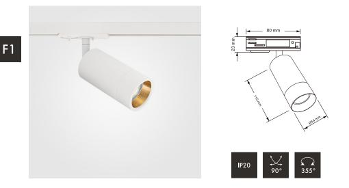
The Shooter L GU10 - is a versatile track mounted spotlight fixture ideal for display and accent lighting purposes. This unit hosts a cylindrical base design, multi directional functions and a set back finish for reduced glare.
