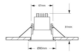
This product is suitable for coverage by thermal and acoustic insulation e.g. loft insulation. Not suitable for blown insulation.
