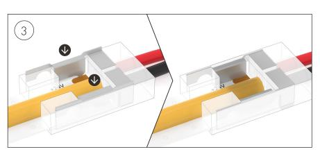
Crimp down on the teeth prongs with pliers to pierce your LED Strip PCB leaving the prongs flush with the connector housing. Check the LED Strip is locked in and the connection is secure.
