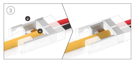
Crimp down on the teeth prongs with pliers to pierce your LED Strip PCB leaving the prongs flush with the connector housing. Check the LED Strip is locked in and the connection is secure.
