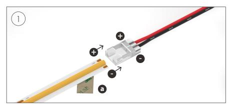
Peel back the adhesive tape leaving a sufficient amount of bare strip to insert into the clip. Make sure you peel back the tape and accompanying adhesive layer leaving this to re-apply once the connection is complete.
