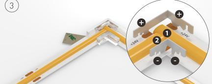
Once LED Strips **1** and **2** are fitted correctly check that the positive **+** copper terminals align with the corresponding clip connector teeth as shown.
