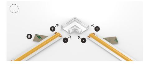
Peel back the adhesive tape leaving a sufficient amount of bare strip to fill the clip. Make sure you peel back the tape and accompanying adhesive layer leaving this to re-apply once the connection is complete.
