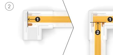
The cutouts within the clip are formed to allow LED Strip **1** all the way into the clip and LED Strip **2** to the position shown.
