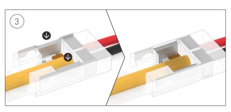
Crimp down on the teeth prongs with pliers to pierce your LED Strip PCB leaving the prongs flush with the connector housing. Check the LED Strip is locked in and the connection is secure.
