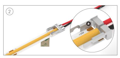
a Insert the LED Strip into the corresponding terminals ensuring the strip is fitted correctly so that the copper pads line up with the clip connector teeth.
