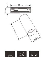
The Shooter GU10 - is a versatile track mounted spotlight fixture ideal for display and accent lighting purposes. This unit hosts a cylindrical base design, multi directional functions and a set back finish for reduced glare.
