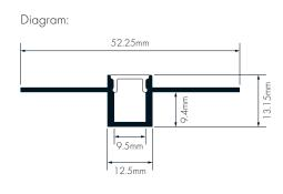
As standard, our Plaster In profiles come with a polyfoam filler designed to simplify installation. Insert the filler into the channel before plastering, leaving one end exposed. Once the plaster has dried, simply remove the filler to reveal a clean, precise finish.
