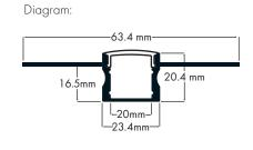
As standard, our Plaster In profiles come with a polyfoam filler designed to simplify installation. Insert the filler into the channel before plastering, leaving one end exposed. Once the plaster has dried, simply remove the filler to reveal a clean, precise finish.
