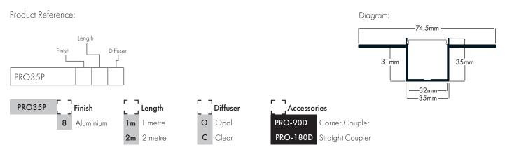
As standard, our Plaster In profiles come with a polyfoam filler designed to simplify installation. Insert the filler into the channel before plastering, leaving one end exposed. Once the plaster has dried, simply remove the filler to reveal a clean, precise finish.
