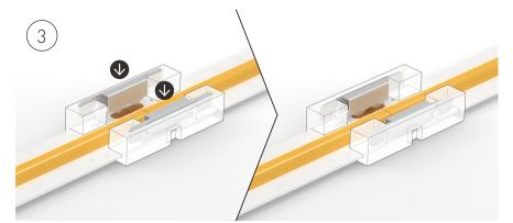
Crimp down on the teeth prongs with pliers to pierce your LED Strip PCB leaving the prongs flush with the connector housing. Check the LED Strips are locked in and the connection is secure.
