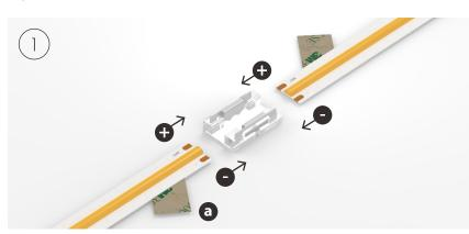
• Peel back the adhesive tape leaving a sufficient amount of bare strip to reach the centre of the clip. Make sure you peel back the tape and accompanying adhesive layer leaving this to re-apply once the connection is complete.
