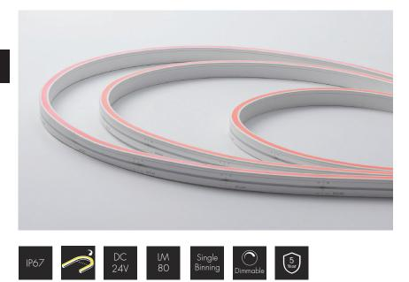
Our LINEAR LED FLEX Side Bend Nano 10w per metre RGB features high efficiency (3 in 1) LEDs on a 2oz PCB board. Housed in a solvent, salt water and UV resistant extruded silicone tube, this product does not require mounting onto a heat sink and offers a LINEAR output in all applications. Side Bend Flex units can be manipulated horizontally up to a 50mm radius with the light source encapsulated along the bottom / top of each run.
