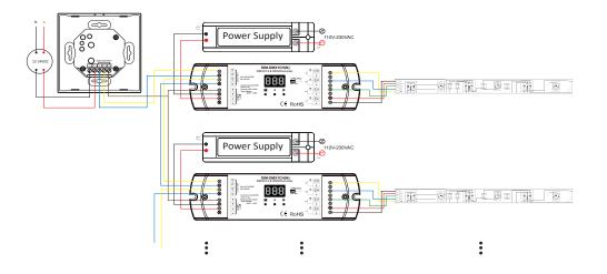
When wiring the decoders, it is important to make sure the total wattage of LED strips doe not exceed the maximum rated wattage per channel. Each channel is rated at 5A, so the maximum wattage per channel is 24x5A=120w.
